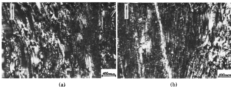
Fig. 4. Effect of capillary length on sample morphology. Longitudinal type A slices, polarized light: (a) sample no. 7, L/d = 21 ; (b) sample no. 6, L/d = 10 .
